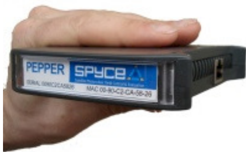
Figure 7: Plug and Play data logger PEPPER counts impulses from a S0 interface and transfers the energy yield with Ethernet connection via internet to the SPYCE server
